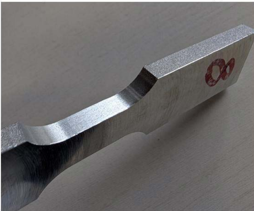
Pic.9. Specimen 8 surface after removal of 0.04mm
