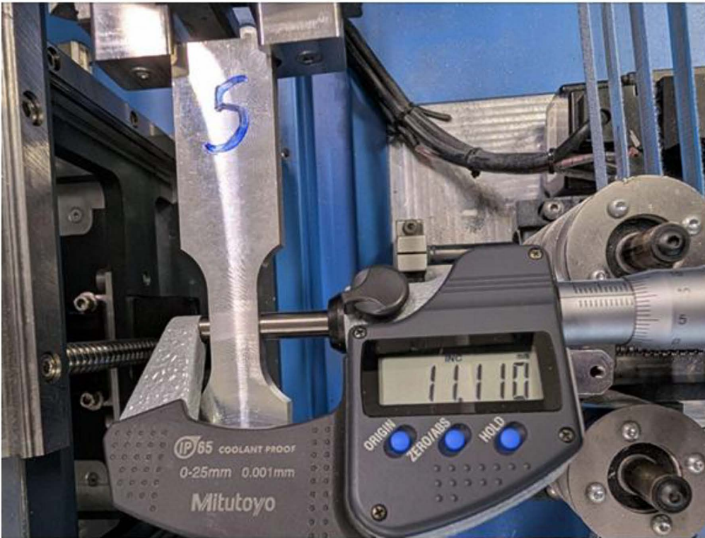
Pic.6. Specimen 5 surface after removal of 0.07mm
