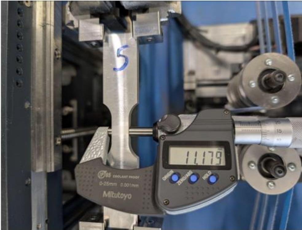
Pic. 2. Specimen 5 "H" - before polishing
