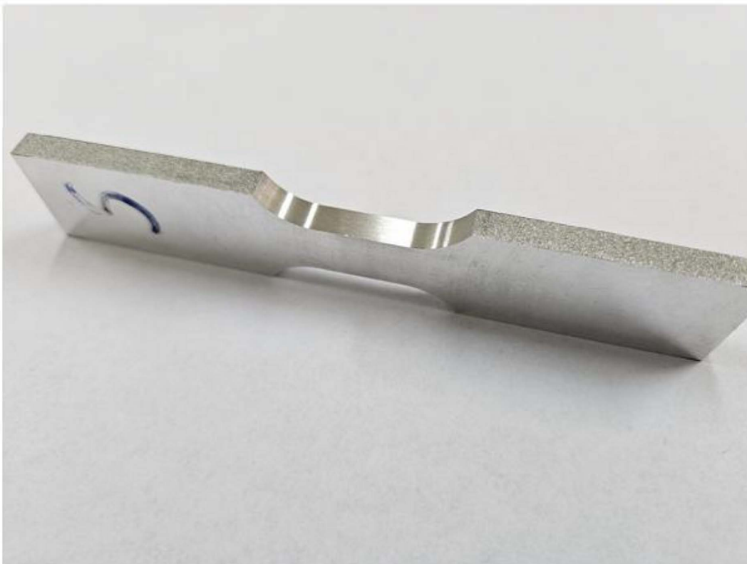
Pic.4. Specimen 5 after step 4 - 0.1mm removal
